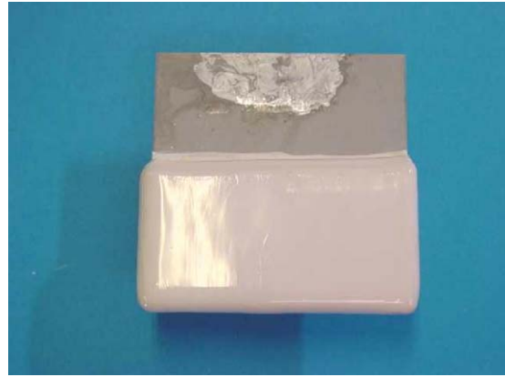
Fig. 7. Green layer fabricated with the following formulation: 90 vol% H 2 O + 10 vol% ethanol, 0.1 wt% of Tiron, 35 vol% of TiO 2 . I_{\text{appl}} = 10 mA.
